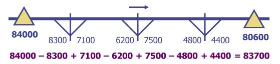
*Figure 1: Example of an imbalance between upstream ATR volume (represented by triangle) and running total of entrance and exit volumes at next downstream ATR.*
